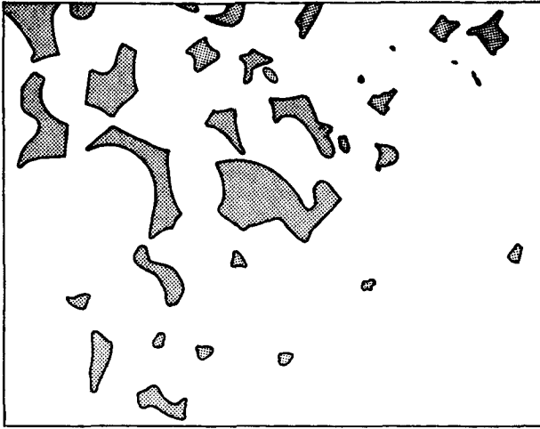
Fig. 1.3 Simplified pore space (black) in a section of smackover carbonate rock.
